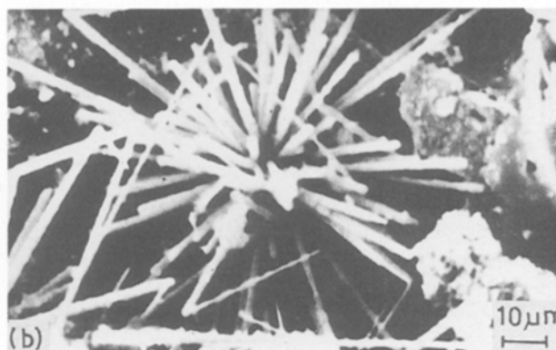
Figure 3 Scanning electron micrographs of ( \text{Si}_3\text{N}_4 plus phenol) compact (core) treated at 1550 °C for 0.5 h. (a) \text{SiC}_w formed in voids; (b) higher magnification of (a).
